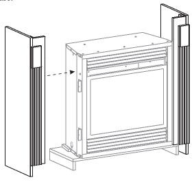
3. Position breastboard assembly to the front of left side assembly and right side assembly.
