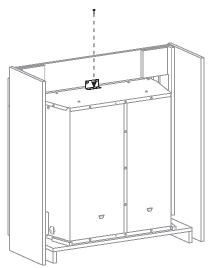
6. Attach back plate to left and right side assemblies through the predrilled holes using the four (4) screws provided, two screws per side.
