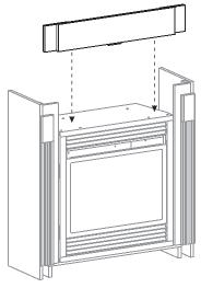
4. Use six (6) 1 1/4" screws to attach breastboard assembly to left side assembly and right side assembly.
