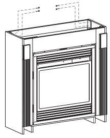
Attach unit to studs in the wall through the "back plate" using two 2 1/2" drywall screws provided.
