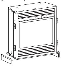
2. Position left side assembly and right side assembly against base.
