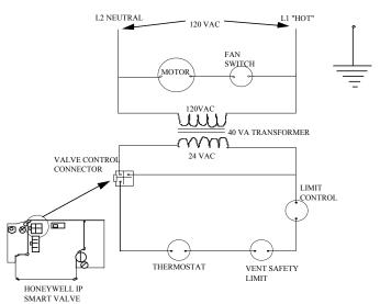
LADDER WIRING DIAGRAM-IP VALVE
