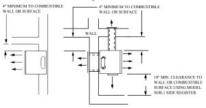
CLEARANCE FOR SIDE OUTLET KITS AND REAR REGISTER KIT TO ADJACENT WALL
