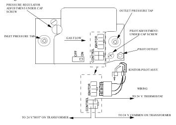
I P-MODEL GAS VALVE AND WIRING
