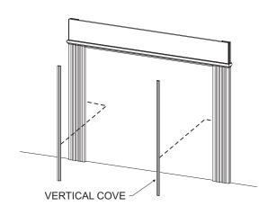
7. Level and attach **top** of 1" X 2" X 42" wall cleat **4 5/8**" above **top** of breastboard to wall with (3) 3" drywall screws.
