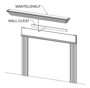
9. Installation of Profile mantel is completed.
