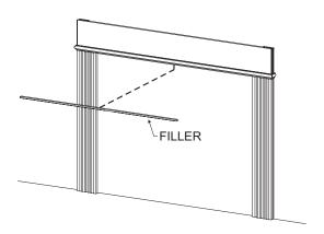
6. Attach vertical cove to inside edge of fluting with finishing nails. The back surface of vertical cove must be flush with front surface of decorative stone or marble. The vertical cove will hold the decorative stone or marble in place.
