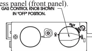
5. Push in gas control knob slightly and turn clockwise to "OFF." Do not force.
