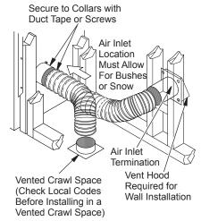
Figure 13 - Outside Air Kit Installation
