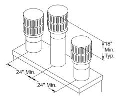
Figure 27 - Multiple Chase Installation
