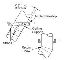
Figure 17 - Chimney Supports
