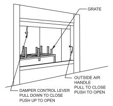
Figure 32 - Damper Operation
