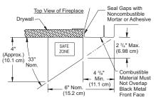
Figure 12 - Mantel Clearances to Metal Face
