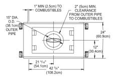
Figure 5 - Framing Clearances
