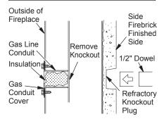
Figure 29 - Gas Line Knockout
