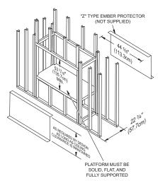
Figure 6 - Framing Firebox with "Z" Type
