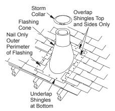
Figure 24 - Flashing Installation
