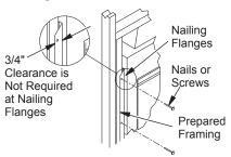
Figure 8 - Nailing Flanges
