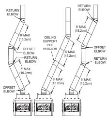
Figure 18 - Typical Offset Installations
