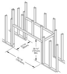
Figure 4 - Framing Firebox
