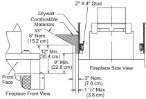
Figure 11 - Mantel Clearances to Combustible Materials
