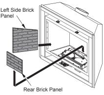
Figure 43 - Installing Rear Brick Panel
