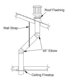
Figure 19 - Offset with Wall Strap and 45° Elbows
