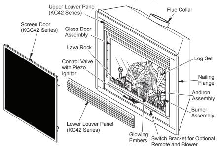
Figure 1 - Direct-Vent Fireplace with Millivolt Ignition
