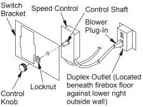
Figure 27 - Attaching Speed Control to Firebox
