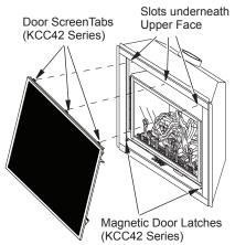
Figure 40 - Removing/Replacing Screen Door Assembly (KCC42 Series)
