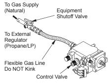
Figure 33 - Connecting Flexible Gas Line to Millivolt Valve
