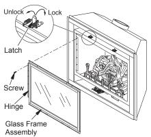
Figure 41 - Removing/Replacing Glass Door
