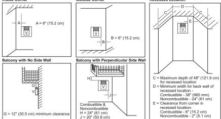
Figure 7 - Minimum Clearances for Termination Cap
