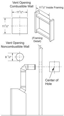
Figure 9 - Vent Opening Requirements
