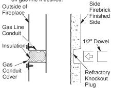
Figure 19 - Gas Line Knockout
