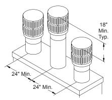
Figure 16 - Multiple Chase Installation
