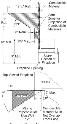
Figure 4 - Mantel Clearances to Combustible Material
