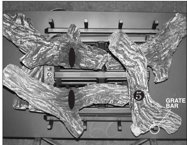
Step (5) Place 'V' area of Log#5 onto grate bar and rest log onto flat area of Log #2.
