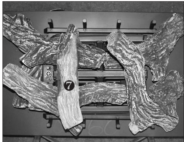
Step (7) Locate notched areas of Logs #2 and 3 and place Log #7 onto these. If sooting occurs on Log #7 it may be removed.
